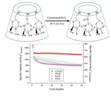
The sulfur utilization and cycling stability of composite cathodes in rechargeable lithium batteries are enhanced by carbonyl- $\beta$ -cyclodextrin (C- $\beta$ -CD) as the binder in sulfur composite cathodes. This is made possible by the fact that C- $\beta$ -CD is highly soluble in water, ca. 100 times more soluble than  $\beta$ -CD at room temperature, and because it exhibits strong bonding strength.
